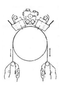
held in both hands. Then the strip is fitted under the brushes (2 or 3 at a time) upside down i.e. abrasive face towards the brush surface and drawn from one side to another. If the brushes have already curved surface this step is not required.
